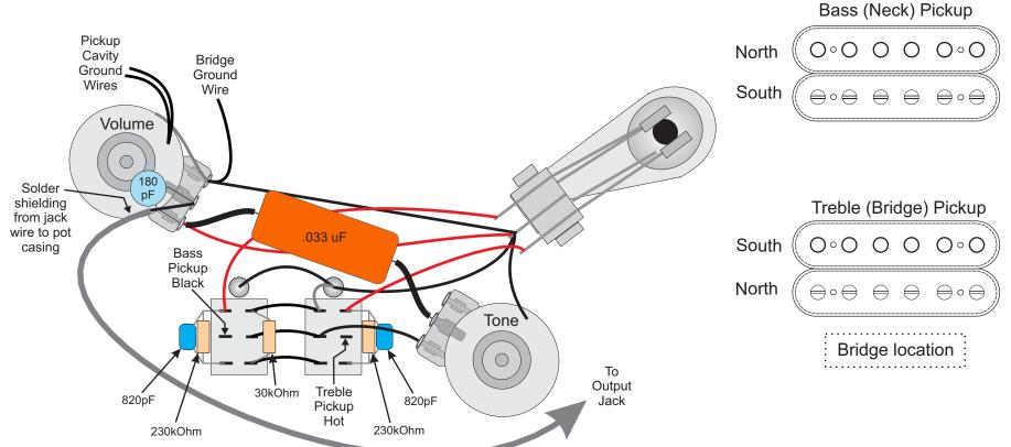
\*Solder bass pickup red and orange and treble pickup harness shielding to volume pot casing
