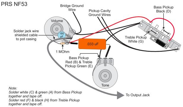
Note Pickup shape is just for reference. All pickups using this diagram shall be oriented in this manner.
