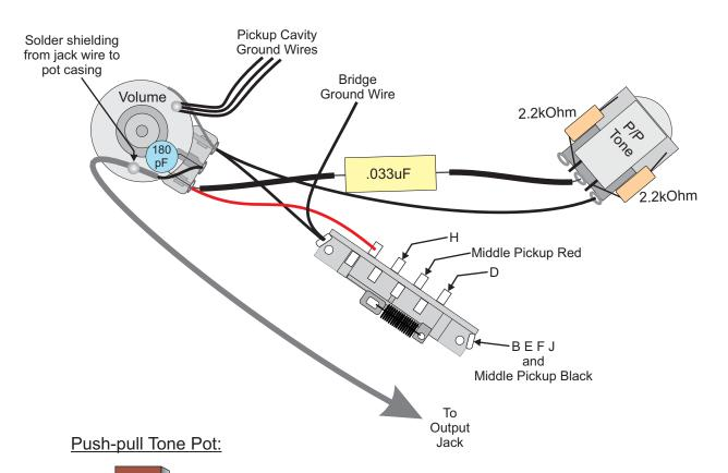
Note: Pickup shape is just for reference. All pickups using this diagram shall be oriented in this manner.
